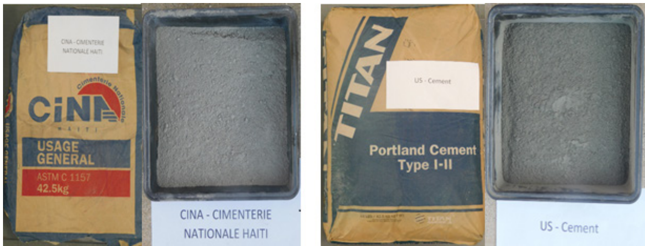
Figure 1: Photographs of cement used on this project; Left Haiti Cement and Right US Cement
