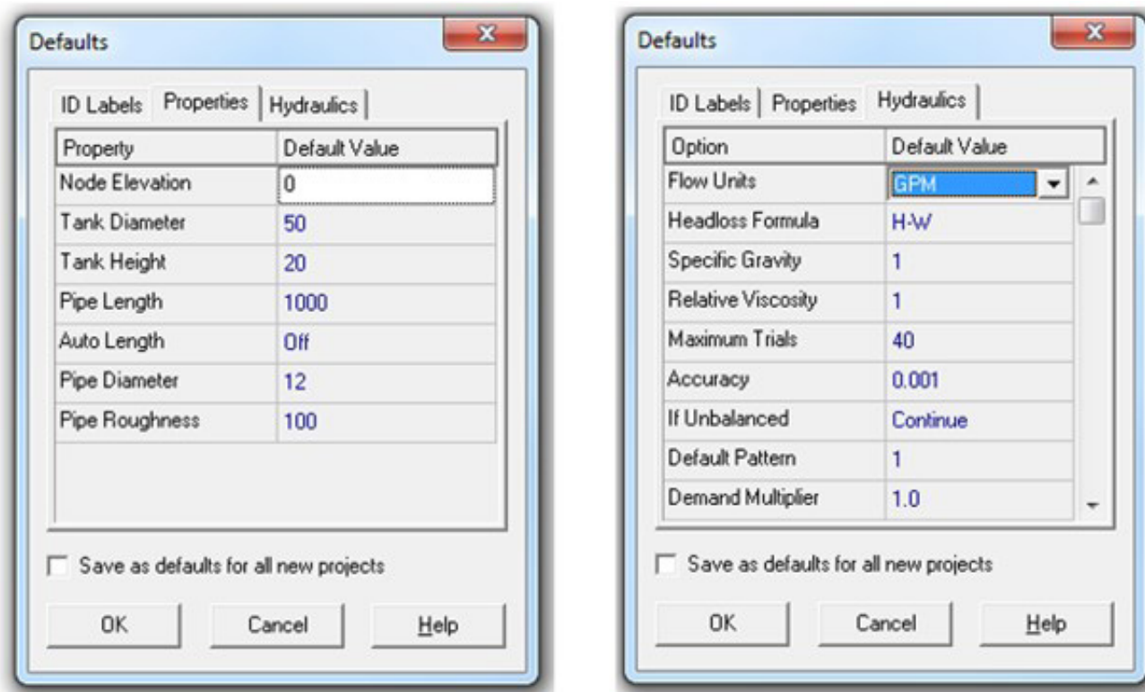
Figure A1: Default properties and hydraulics when setting up an EPANET model
