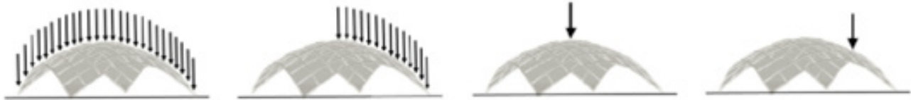
Figure 4: (left to right) Load cases – symmetric distributed load, asymmetric distributed load, centred point load, off-centred point load
