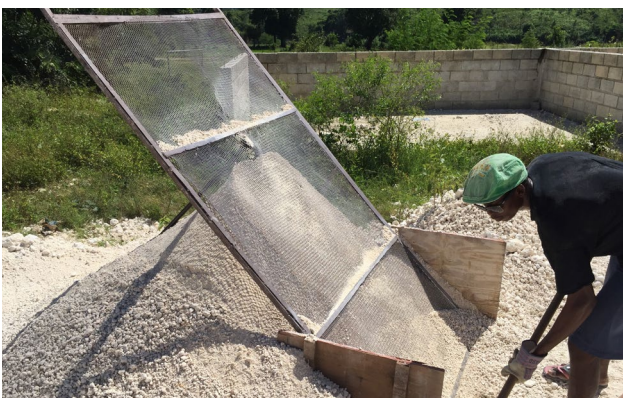
Top to bottom: Figure 1. Clemson engineering students with CMU plant employees Figure 2. The quarry where aggregate and sand are excavated Figure 3: Process flow diagram of CMU manufacturing plant in Haiti Figure 4: An employee sieving aggregate with a shovel
